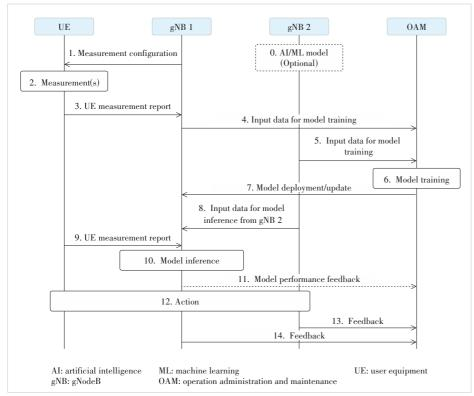
▲ Figure 3. Deployment of AI/ML functionality: model training at OAM and model inference at nextgeneration radio access network (NG-RAN)
