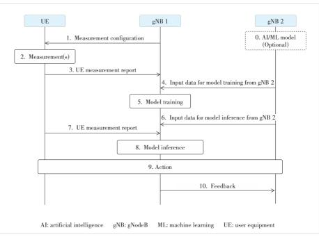
▲ Figure 4. Deployment of AI/ML functionality: model training and model inference at nextgeneration radio access network (NG-RAN)
